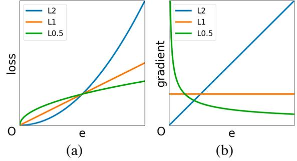
Figure 7. **Comparison of different norms.** (a) Different norm-based losses about  $e$ . (b) The gradient of different norm-based losses with regard to  $e$ . The horizontal axis  $e$  denotes the pixel-wise distance of image reconstruction with the estimated reference image depth. The  $\mathcal{L}2$  norm aims to reduce outliers, the  $\mathcal{L}1$  norm treats all points equally, while the  $\mathcal{L}0.5$  norm concentrates more on accurate points.
