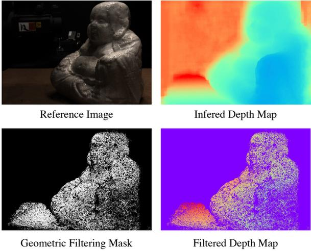
Figure 6. **Depth filtering.** Most points with inaccurate depth will be filtered out before depth fusion. It can be observed that these points usually locate in occluded regions or useless backgrounds, where photometric consistency fails.
