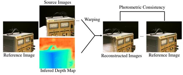
Figure 3. **Photometric consistency.** The source images are warped to reconstruct the reference image with the inferred depth map on the reference view. Then consistency is enforced between the reconstructed images and the reference image.
