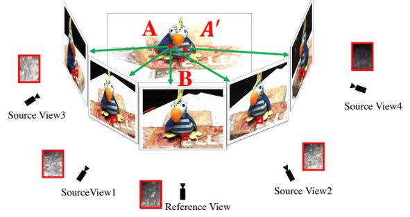
Figure 5. **View-dependent effects and occlusions.** From source view4, point  $A$  is occluded and only point  $A'$  is visible along the line of sight. Besides, The appearance of the identical region  $B$  differs in different views due to variations in illumination, camera exposure, and reflections.
