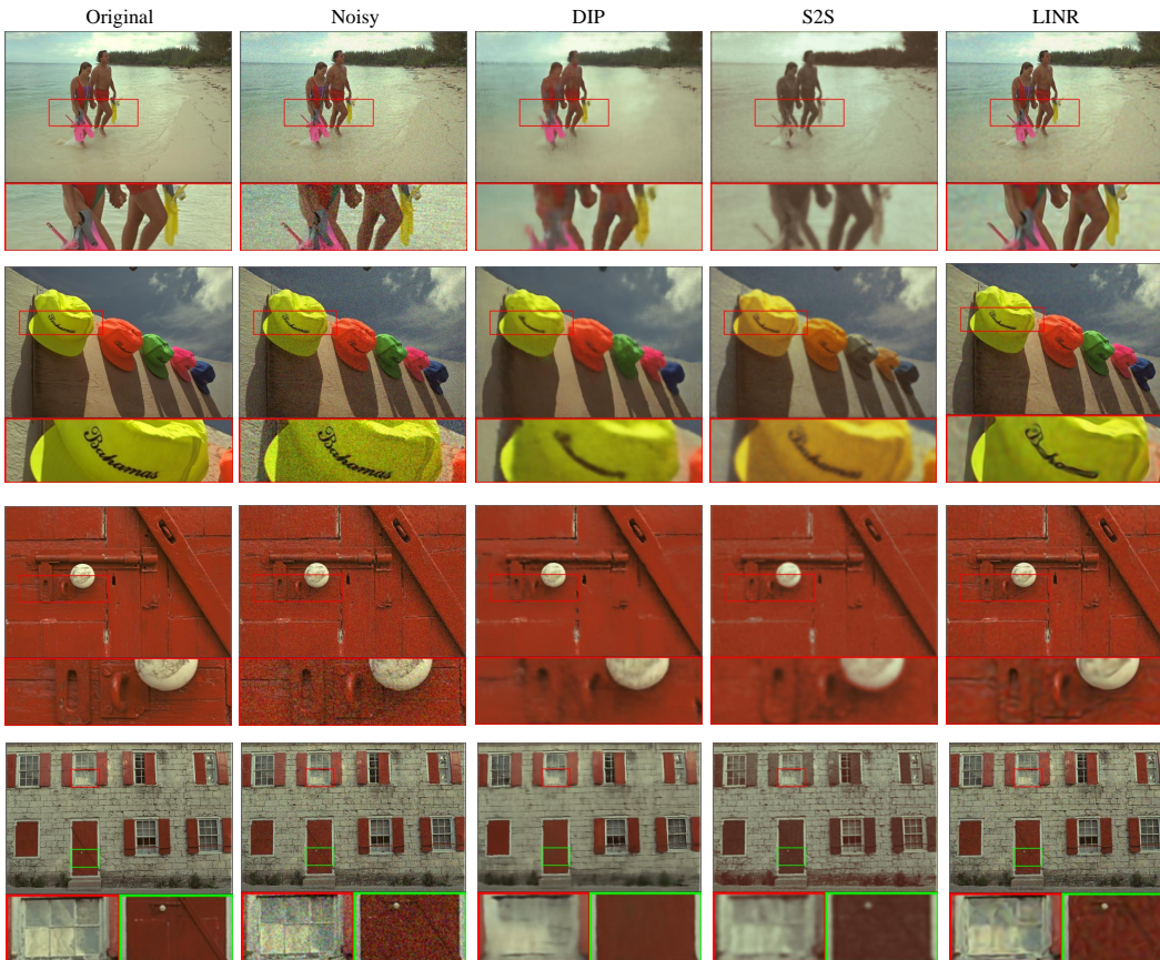
Figure 12: Qualitative results on denoising with \sigma = 25 . LINR 's denoise results contain more detailed information than other methods.
